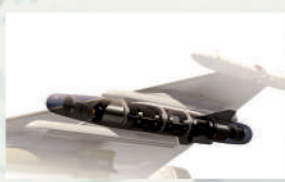
RWR / JAMMER PODS Sensor : EW System
