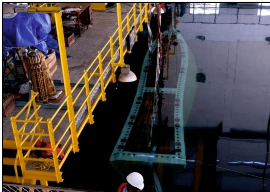
Indigenous Bow-Mounted Dome Undergoing Acoustic Tests at NPOL 54 Breakthrough with the Induction of INS Sagaradhwani
